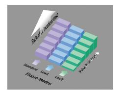
**3-dose mode** control allows a choice of 3 customized dose modes and 6 fluoroscopic pulse rates of up to 30 f/s to optimize the fluoroscope image while realizing the most effective dose reduction.
