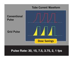
**Grid pulse fluoro** features in-tube grid switching that virtually eliminates leading and trailing edge dose for more efficient pulse fluoroscopy.
