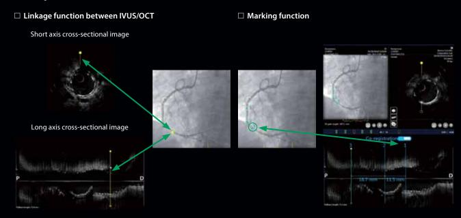
There are two main functions in IV-LINQ. The first is co-registration of IVUS/OCT with the angiographic image. Once registered, the IVUSOCT position (both short and long axis) can be determined relative to the angiographic image. The second function is the ability to annotate the image with markers, facilitating stent planning and placement.
