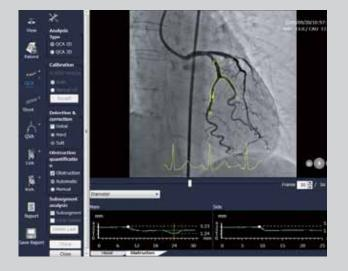
QCA\* features automatic contour detection and analysis of the area of interest. Various calibration options are available, such as Catheter, Sphere, and Distance calibration methods.
