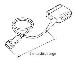
Never immerse the non-waterproof sections of the transducer into liquids such as water or cleaning solution. Immersion may cause electric shock.
