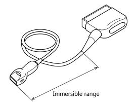
Never immerse the non-waterproof sections of the transducer into liquids such as water or cleaning solution. Immersion may cause electric shock.
