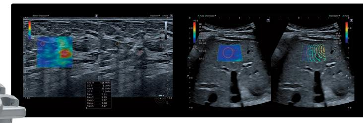
Canon's shear wave technology provides a quantitative measure and realtime display of tissue elasticity in a variety of clinical settings ranging from abdominal to small parts examinations. Smart Maps help you visualize and quantify shear wave propagation in realtime. Aplio's unique propagation map is a powerful and intuitive tool to visually assess the quality of an elastogram.
