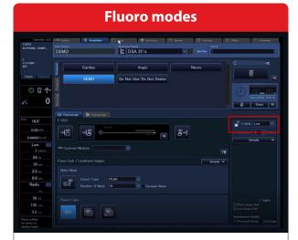
Variable dose modes to pre-programmed combinations of pulse rate, dose level and image processing parameters
