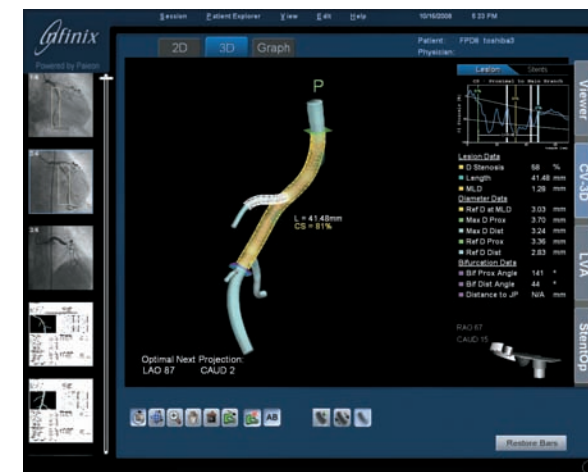
The CV-3D workstation works with the Infinix-i to transform 2D imaging into a 3D display for coronary vessel analysis showing coronary vessel and side branches with stent placement modeling (left: stent planner) and an enhanced view (stent optimizer) of a stent after placement.
