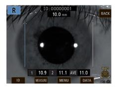
Diameter measurement of the pupil, cornea or contact lens can be performed.
