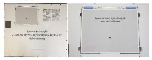
2. Please make sure to cover the battery pins to avoid liquid entering in to sensor panel.
