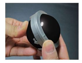
NOTE: Be sure to insert the inner ring when setting the ball. If the inner ring is not fitted properly, the ball may not rotate properly. Be sure to fit the inner ring properly.
