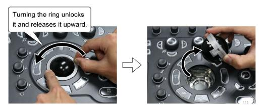
*NOTICE:* To prevent malfunction, be careful when removing the ring.
