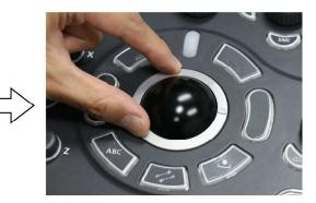
(g) Turn the ring in the direction of the arrows until it is locked (fixed).
