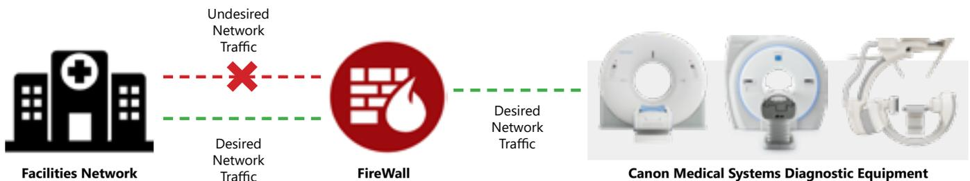
For customers that are not currently under Canon Medical Systems USA warranty or service agreement, Canon Medical offers a vendor and modality neutral firewall appliance called eProtect to isolate and secure any diagnostic imaging equipment from undesired network traffic. eProtect is an external hardware appliance residing in series of the diagnostic equipment and the facility network.
