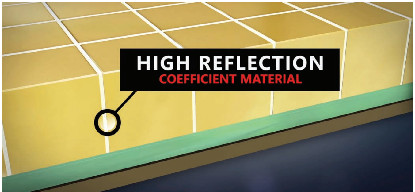
Figure 5 Highly reflecting material between detector elements minimizes detector cross-talk to maintain superior spatial resolution and avoid signal loss.
