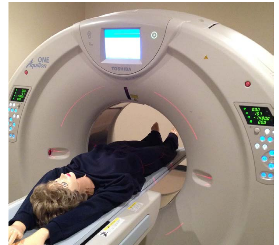
Figure 3: An anthropomorphic phantom was scanned at multiple table heights to demonstrate the benefit of positioning compensation technology.
