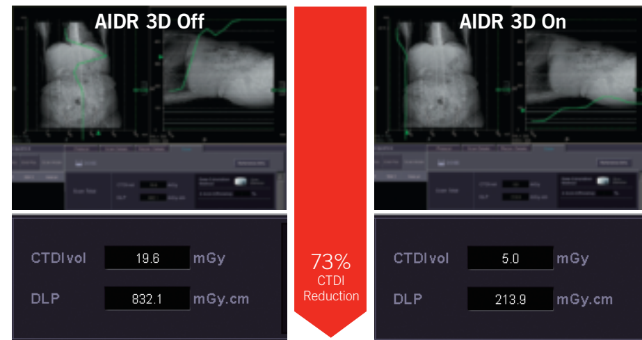
Figure 9: Example of SURE Exposure integration: Prior to scan, AIDR 3D was toggled off (left) and on (right) in the protocol to demonstrate how SURE Exposure automatically reduces the tube current (see green mA curve), thus lowering the dose (CTDI) automatically.
